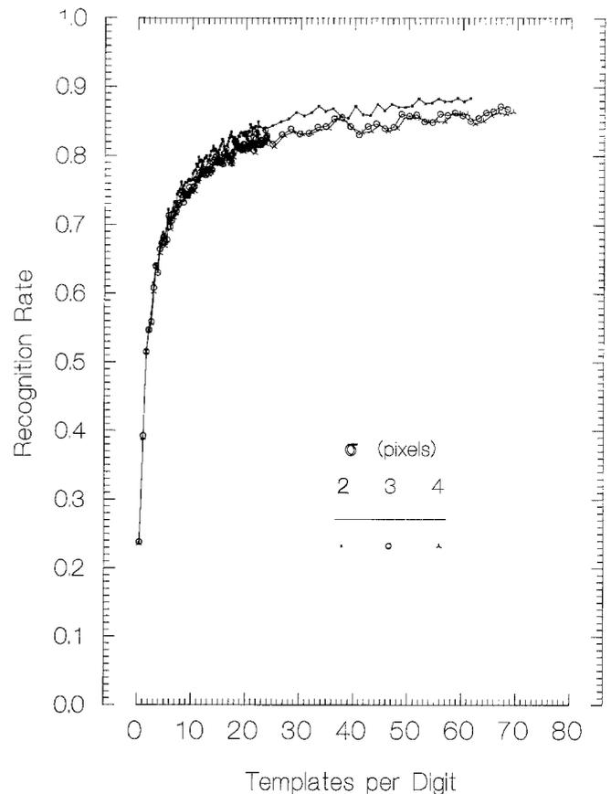
**Fig. 4.** Mean rate of recognition compared with mean number of templates per type of digit for successive blocks of trials in the seven conditions of Experiment 1. The Gaussian smoothing parameter  $\sigma$  was varied between conditions. Left panel: Results for  $\sigma = 0, 0.5, 1,$  and
