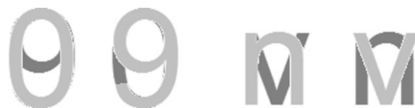
Fig. 2. Illustration of physical overlap (cross-correlation) between symbols. On the left we have overlaid an Arial font '9' (dark grey) on '0', and '0' (dark grey) on '9'; these symbols have a very high cross-correlation of 0.85. On the right an illustration of overlaying 'v' (dark grey) with 'n', and 'n' (dark grey) on 'v', respectively; these two letters have a quite low cross-correlation of 0.37.
